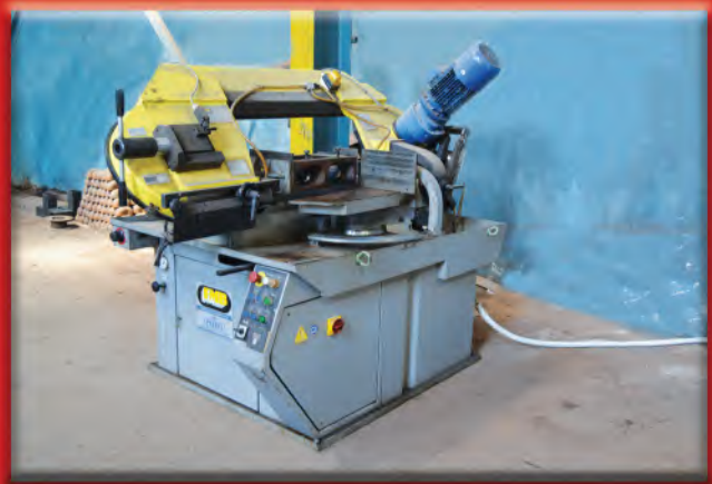
Saw Zall ( profiles & Pipes Cutting )
