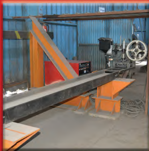
Submerge Automatic Welding Machine ( For Builtup Welding ) Length 18 meter
