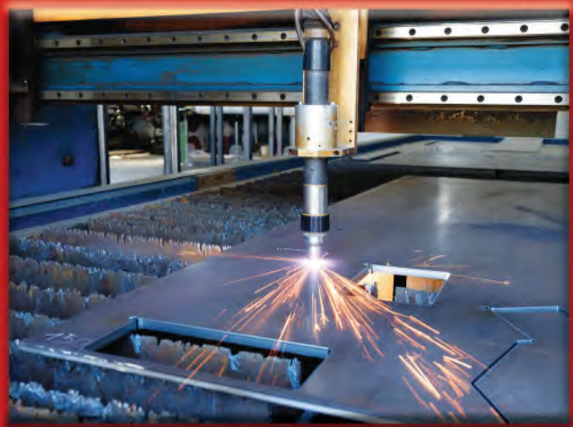
CNC Plate Cutting( 2.5x12 Meter ) ( Plasma & Oxy fuel )
