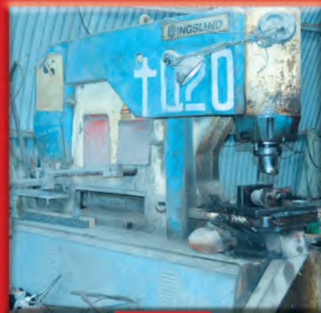
Punch (Cutting Profiled - Predding holed - Slots )
