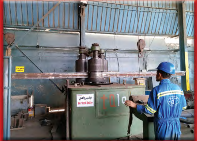
Profile Rolling Machine ( Beams , Angles , Pipes )
