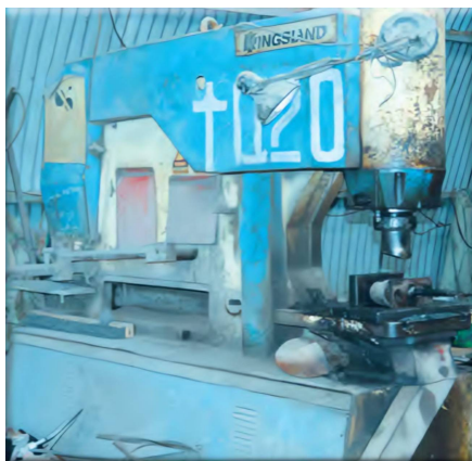
PUNCH • PROFILES, HOLES, SLOTS
